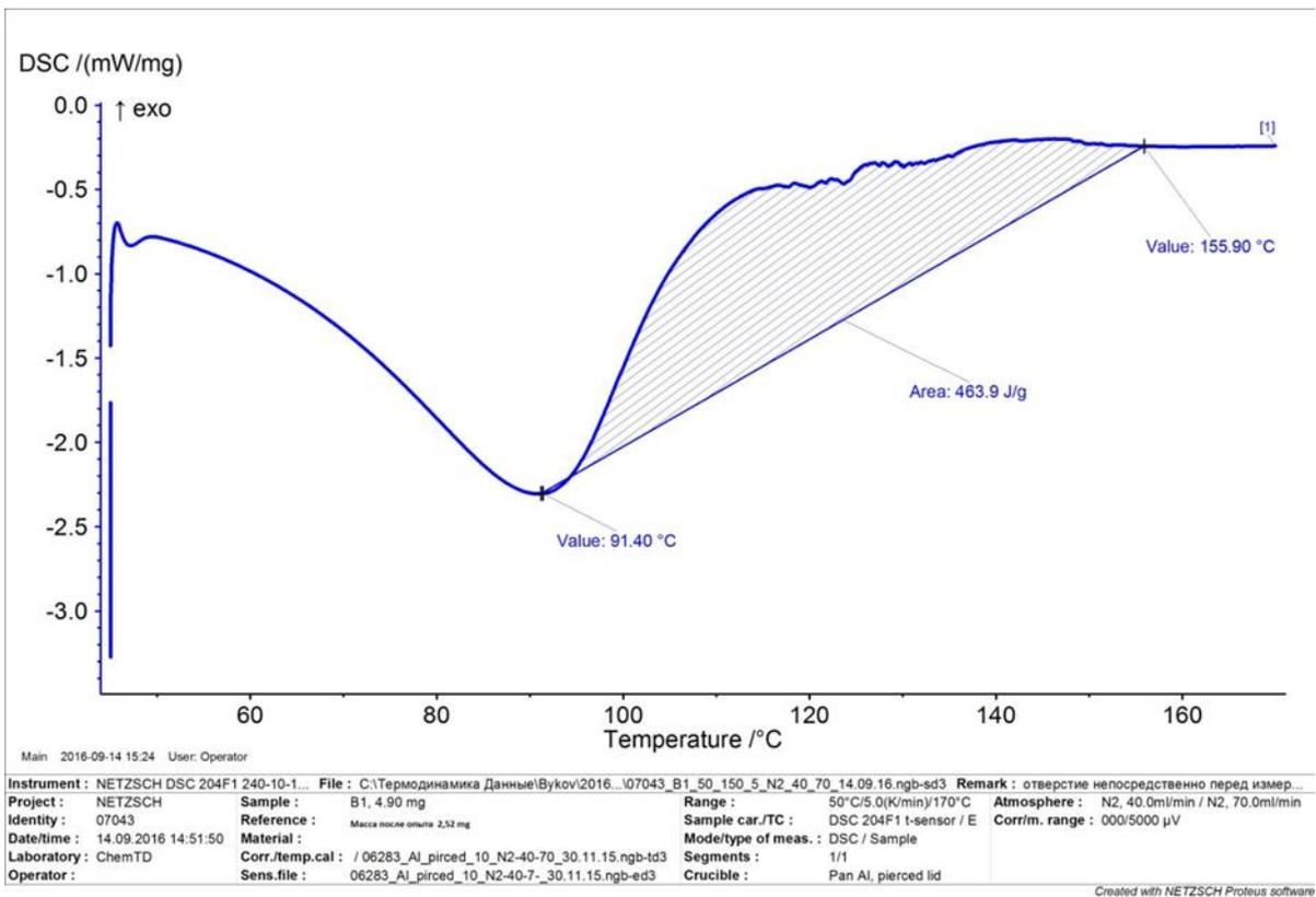
Pic. 3. Thermal data of the heating of pure binder from 25°C up to 170°C (experiment with binder dd. 14.09.2016).
