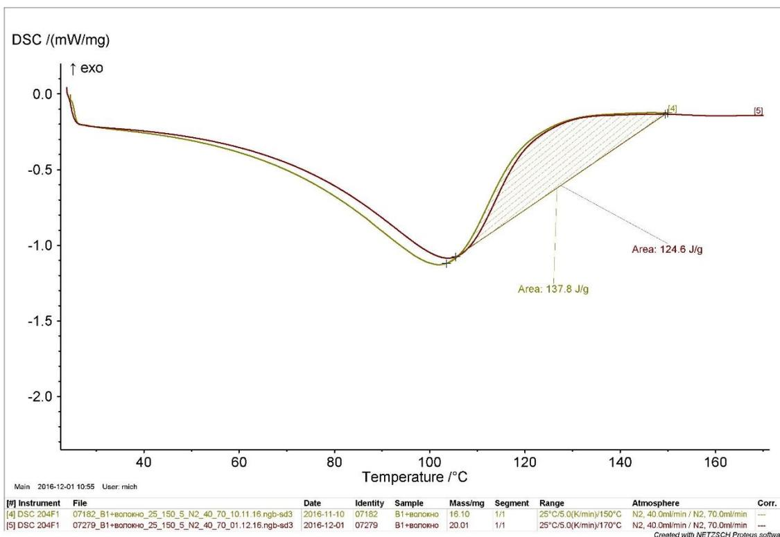
Pic. 1. Thermal data of the heating of binder with fibre. The temperature range is between 25°C and 150°C (grey curve, experiment dd. 10.11.20016) resp. 170°C (purple curve, experiment dd. 01.12.2016).
